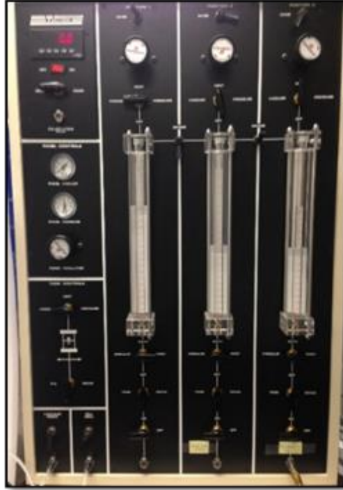
Figure 3-6. Pressure control panel (Trautwein soil testing Co.)
