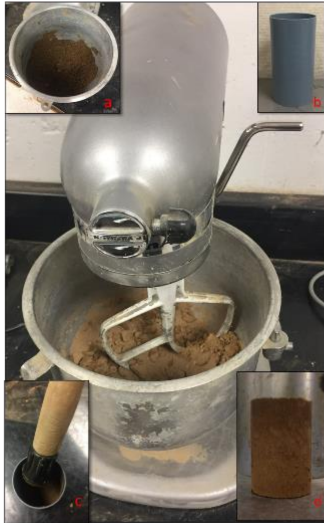
Figure 5-1. Procedure of making S/S specimen
